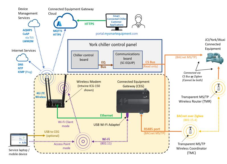
Figure 1.1.1 above reflects a scenario with Johnson Controls only devices such as York and Wuxi connected equipment. The CS bus is active on the SC-EQUIP board, while the BAS Port / FC bus is not used to connect chiller equipment. Optionally, the BAS Port / FC bus may be used for Metasys connectivity independent of the connected solution.
