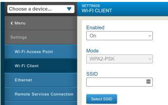
d. In the field "Client SSID", enter the SSID of the wireless network that the CEG will be connecting to. In the field "Passphrase", enter the passphrase for the wireless network the CEG will be connecting to.
