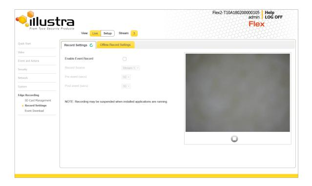
By utilizing SD card storage, if a network video recorder goes offline, the camera has the ability to record some amount of video internally.
