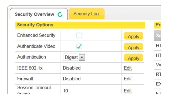
The Digest authentication means that the username and password being passed in the RTSP authentication of the video is not passed in clear text. Basic authentication does not protect the transmission of the username and password and is not recommended.
