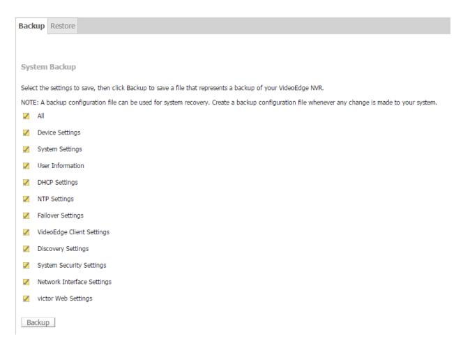
While Operating System (OS) settings cannot be stored in the configuration backup file, the system will automatically export a text file containing the OS settings once you click the back button. The text file can be used as reference for manually configuring the OS settings.
