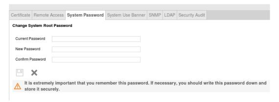
**Note:** It is critical that the new password be recorded and kept secure as it cannot be recovered. The web UI has a warning to this effect.
